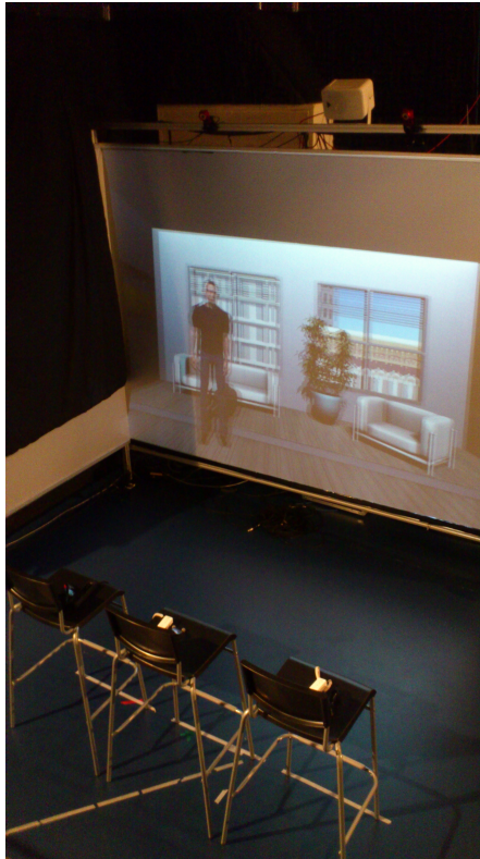
Figure 8.4: Photo of the experimental setup showing the three bar stools and a projected s-3D image.
