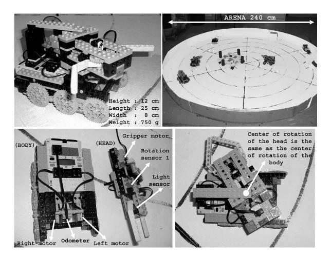
Figure 1: Robots and environment
