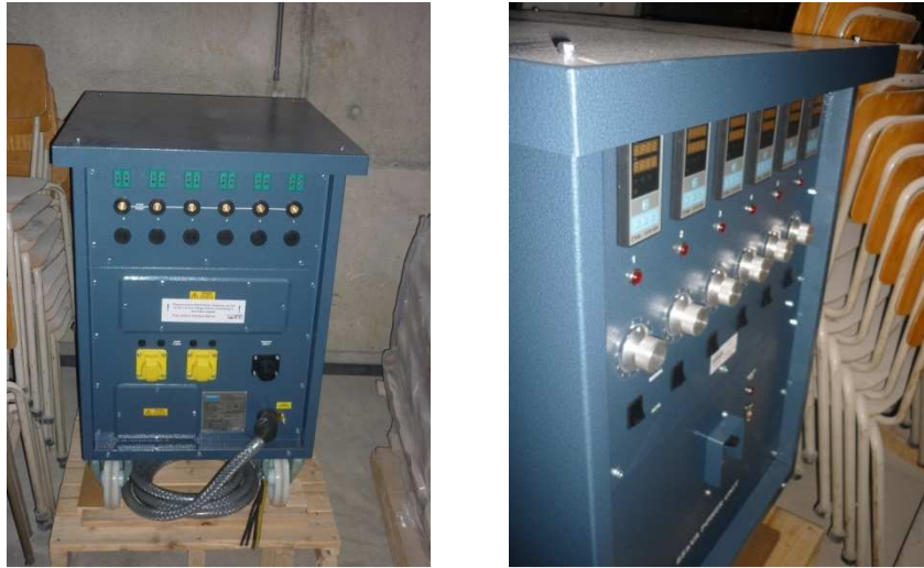
Figure 21 : Mannings 65kVA power unit with 6 temperature controllers
