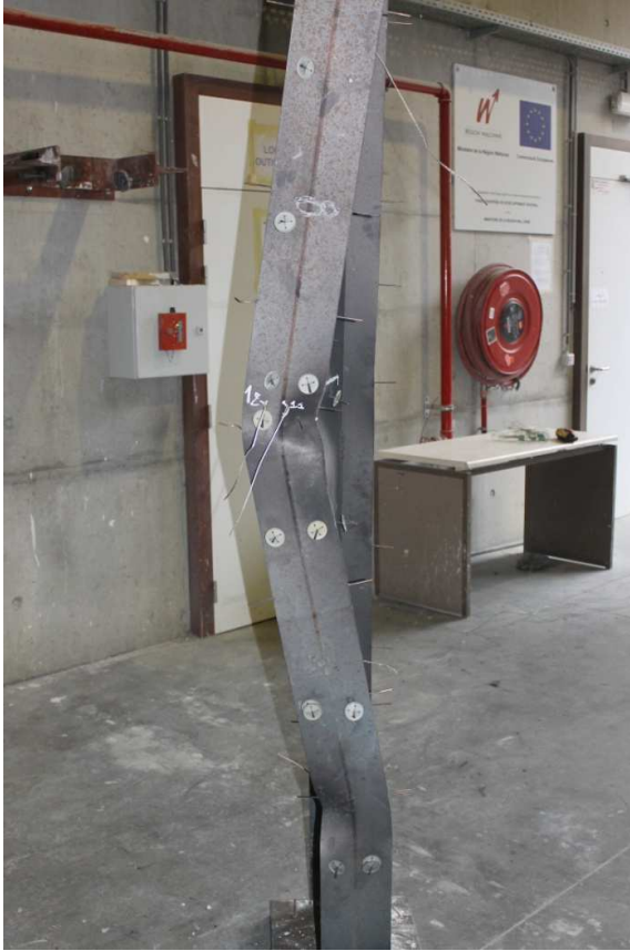
Figure 84 : Test No 8: Deformed shape of the column after the test
