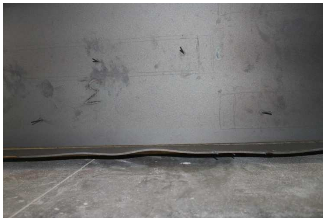
Figure 59 : Test No 3: Deformed shape of the column after the test
