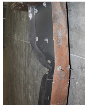
Figure 74 : Test No 6: Deformed shape of the column after the test
