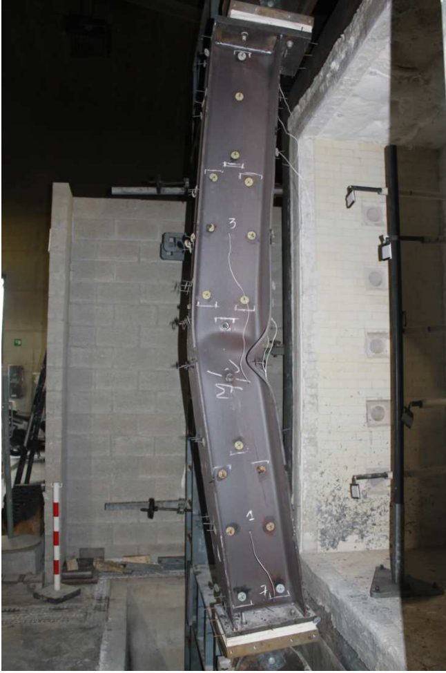
Figure 79 : Test No 7: Deformed shape of the column after the test
