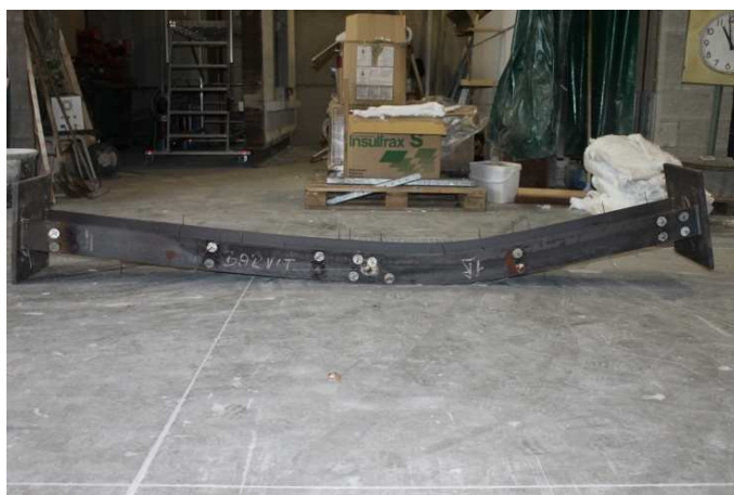
Figure 49 : Test No 1: Deformed shape after the test
