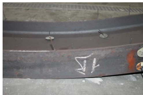
Figure 49 : Test No 1: Deformed shape after the test
