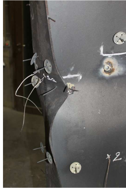
Figure 84 : Test No 8: Deformed shape of the column after the test
