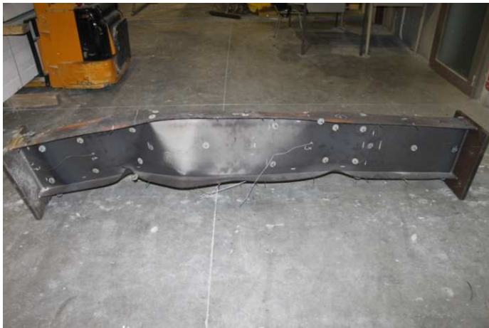
Figure 69 : Test No 5: Deformed shape of the column after the test
