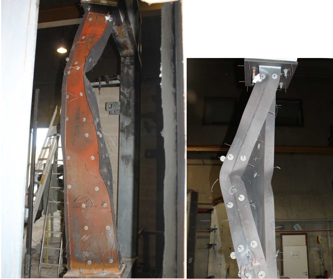
Figure 64 : Test No 4: Deformed shape of the column after the test
