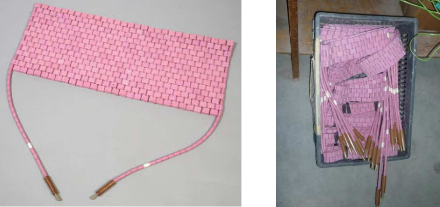
Figure 23 : Ceramic pad heating elements
