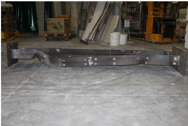
Figure 74 : Test No 6: Deformed shape of the column after the test
