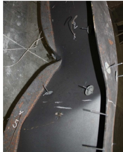
Figure 69 : Test No 5: Deformed shape of the column after the test
