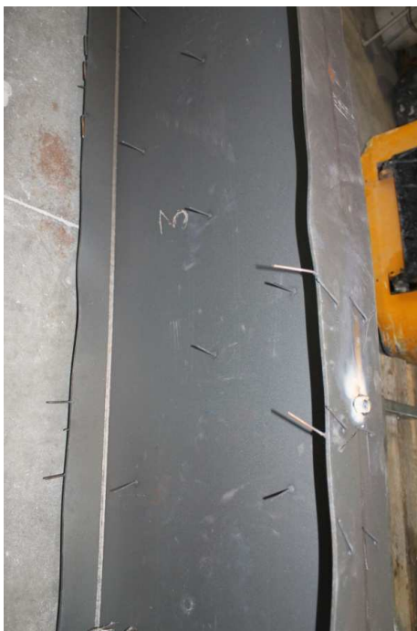
Figure 59 : Test No 3: Deformed shape of the column after the test
