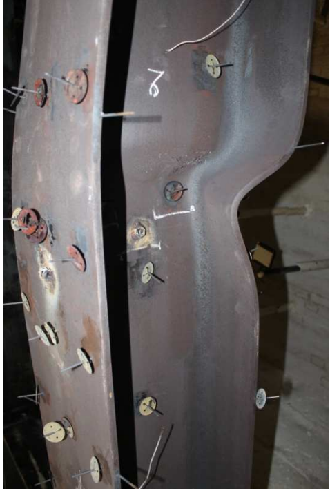
Figure 79 : Test No 7: Deformed shape of the column after the test
