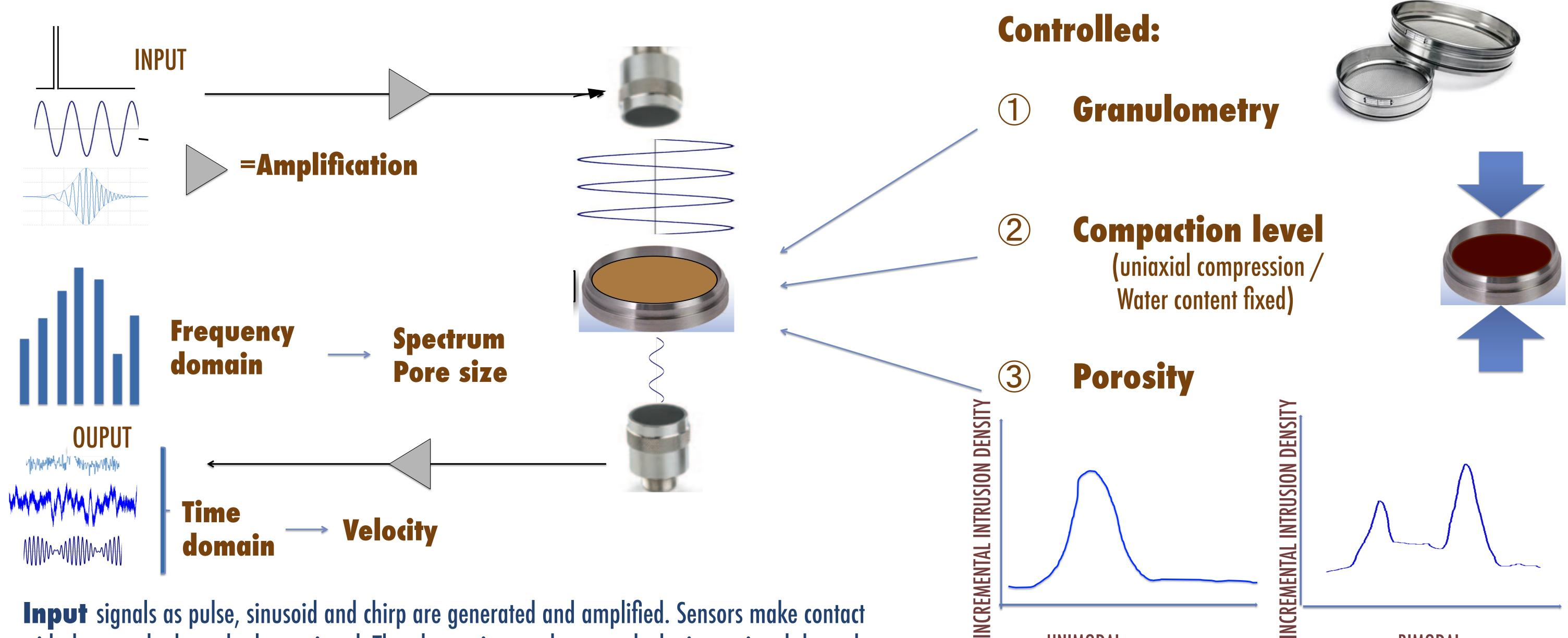
**Input** signals as pulse, sinusoid and chirp are generated and amplified. Sensors make contact with the sample through ultrasonic gel. The ultrasonic transducer sends the input signal through the sample. The attenuated signal is received by the opposite piezoelectric sensor. Finally, the signal received is amplified and digitized. All the acquisition is controlled with labview. Output signals are treated and postprocessed using Matlab.
