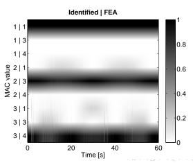
The mode shapes are perturbed by the presence of the mass on the beam
