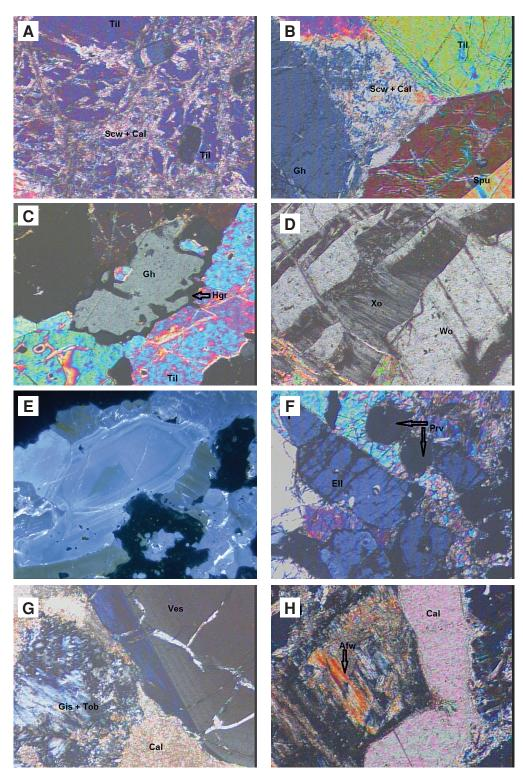
Cathodoluminescence (CL) analyses were performed on thin sections using a Technosyn 8200 Mark II coldcathode electron gun mounted on a polarizing microscope. The electron beam was accelerated at 10-15 kV, with a 400-500 mA beam current.
