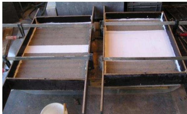
Figure 28 : Slabs repair preparation (EPS defects)
