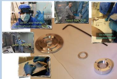
Figure 4: Mounting of the AGPM in the Paranal clean room. The component, which looks like a tiny compact disk (10 mm diameter and 0.3 mm thickness), was handled with care and inserted into a dedicated mount (designed in Belgium by GDTech to support a cool down from room temperature to a few tens of Kelvin). The assembly was then mounted onto the "slit/mask" wheel (focal plane) of CONICA.
