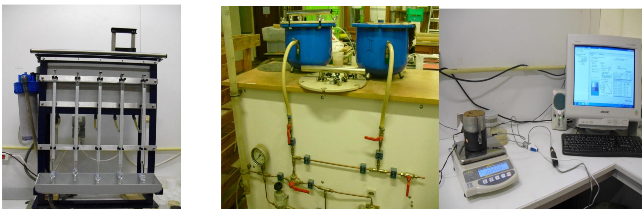
Figure.1. Classical methods to measure soil water retention and hydraulic conductivity
