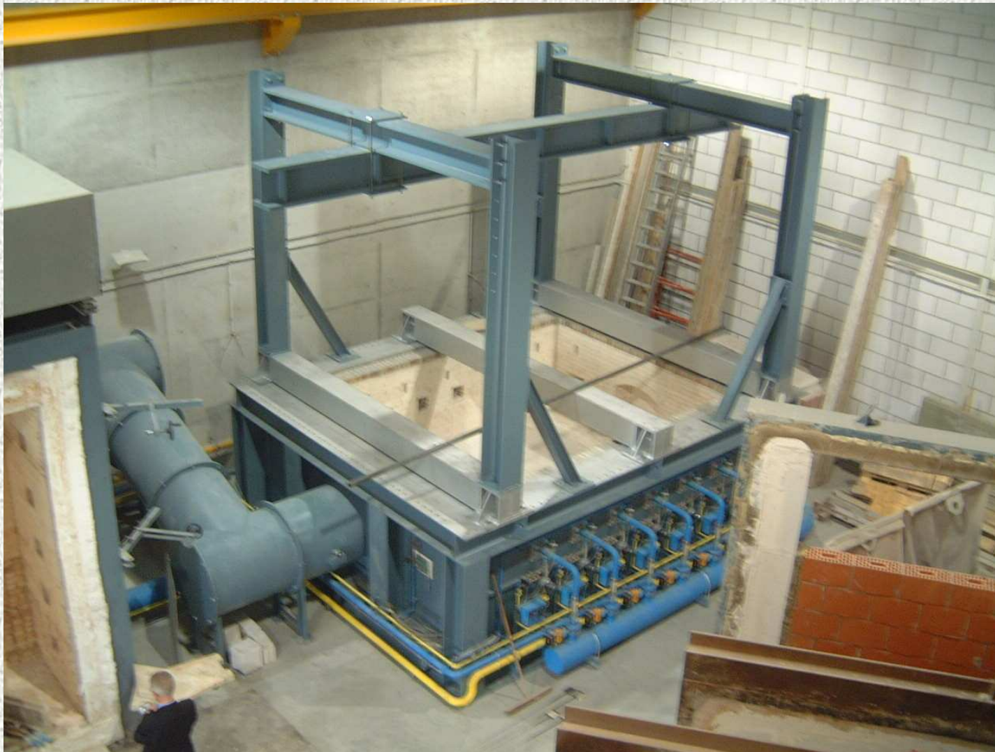
Horizontal (and multi-purpose) furnace (3x4 m 2 ) with loading system (1000 kN)
