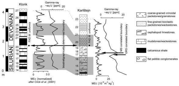
Fig.1. The MS and GRS stratigraphic correlation of the GSSP Klonk and parastratotype at Karlštejn. Note variable position of the S-D boundary at Karlštejn determined by biostratigraphic indicators and combined MS and GRS.
