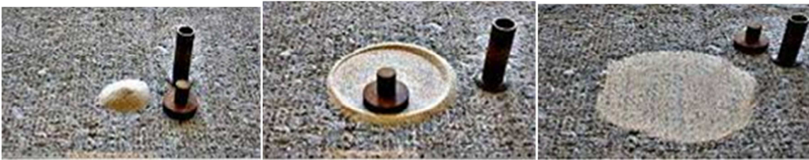
Fig.2. Sand test for surface roughness evaluation
