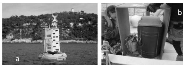
Fig. 1. Picture of the EOL Buoy (a) and of the cytometer installed on it (b)
