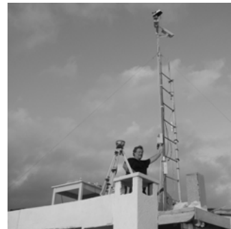
Fig. 2. Monitoring system, meteorological station and D-GPS station, installed on-site.
