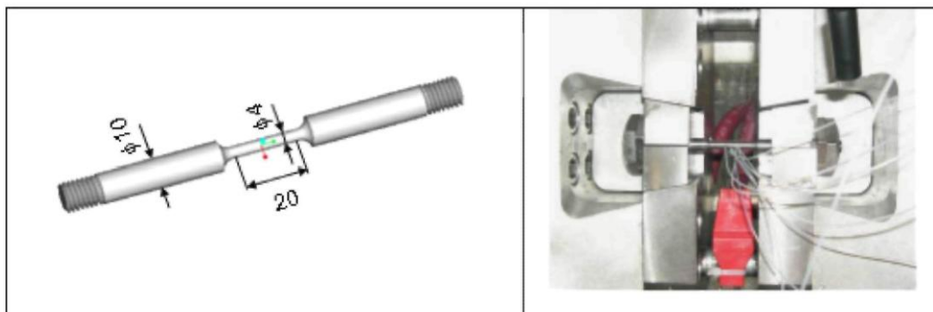
Fig. 2. Tensile specimen (dimensions in millimeter) and testing apparatus on Gleeble™ 3800.
