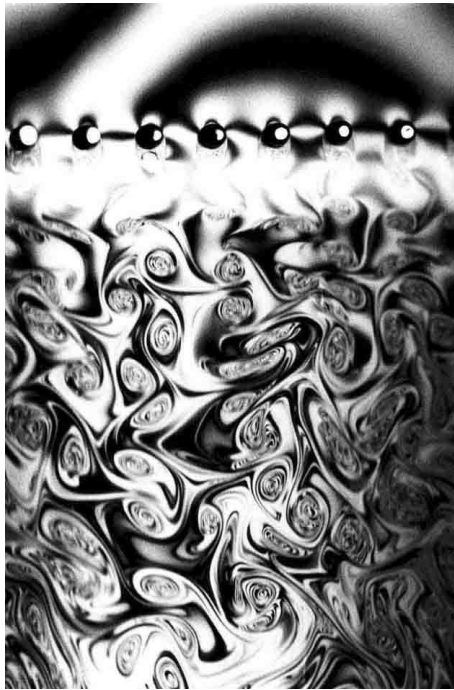
Figure 1.18: Picture of the wake below a comb set into a flowing soap film (from [51]) The visualization of the interference pattern is obtained by lighting the film with monochromatic light (Sodium lamp).
