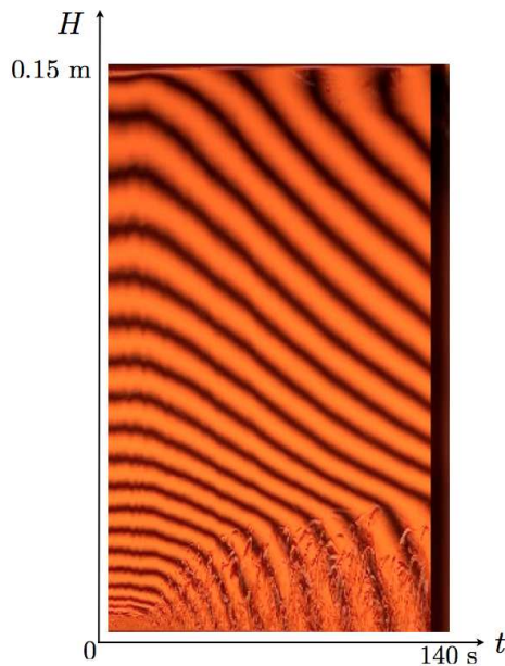
Figure 2.2: Spatio temporal diagram of the fringe pattern of a freely suspended vertical soap film. The black area for larger times corresponds to the film rupture.
