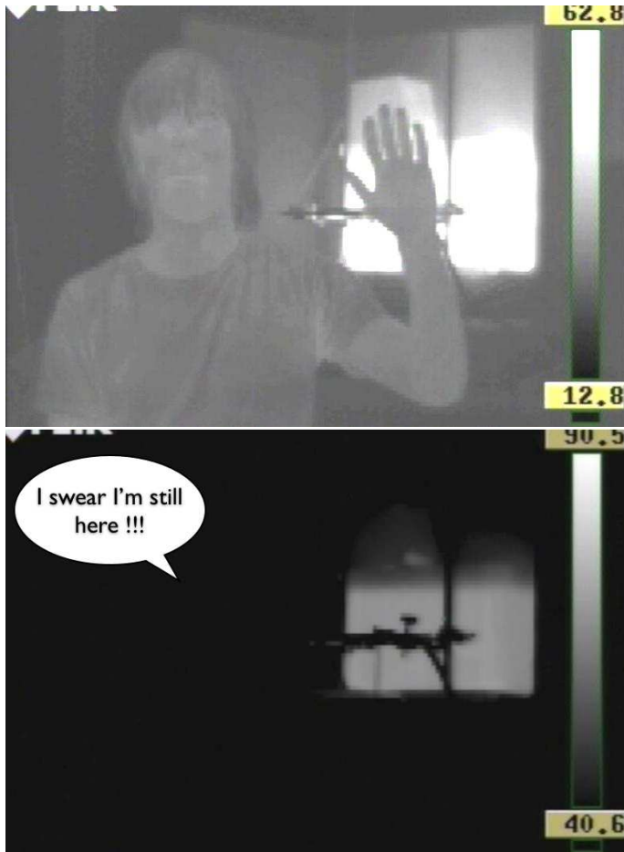
Figure 2.8: Examples of infrared images obtained by the thermal camera. Up : this image is built with a level of 25^{\circ}\text{C} and a range of 50^{\circ}\text{C} . The settings of the camera are so that the thermalized bath, the lab environment and the experimenter are displayed. Down : the same situation filmed with a level of 65.5^{\circ}\text{C} . Only the thermal bath is visible with these settings. The lab environment and the experimenter, though still present, are not displayed.
