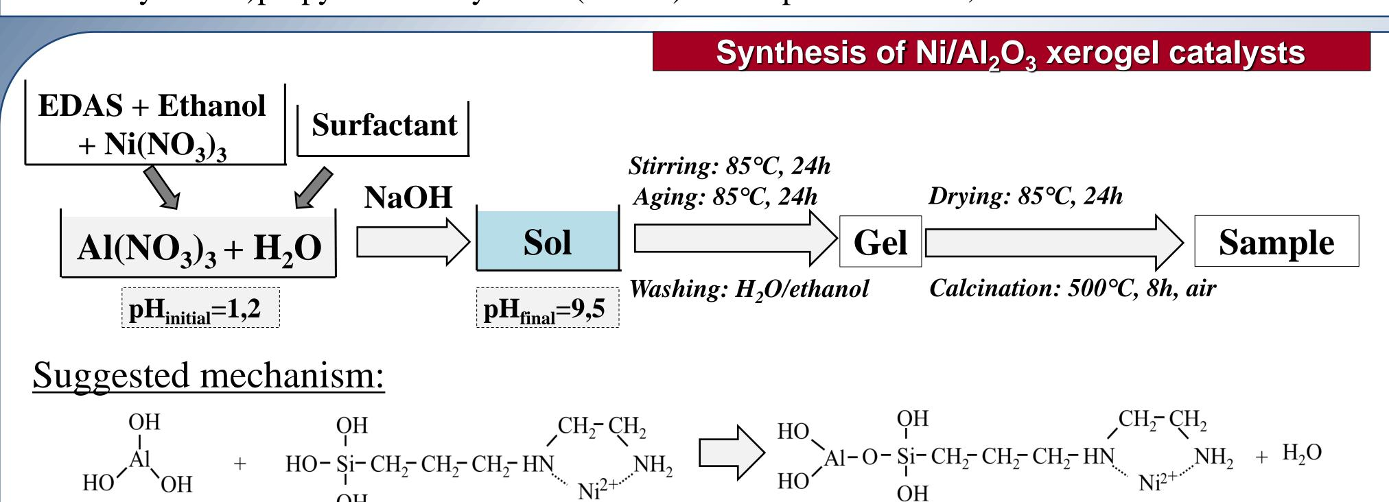
The complexation of Ni<sup>2+</sup> ions by EDAS allows to disperse homogeneously, after calcination and reduction steps, Ni
