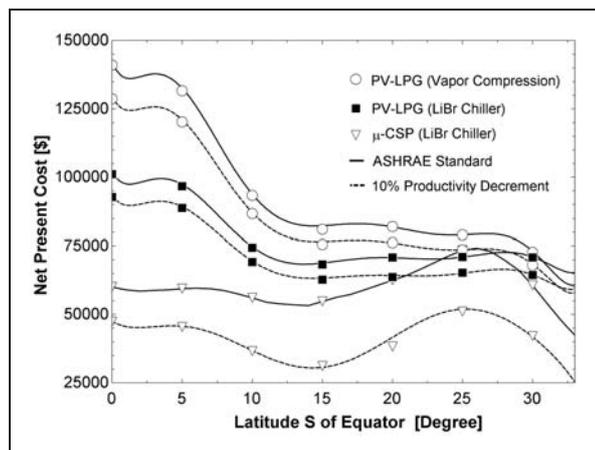
**Figure 7.** Variation of Net Present Cost (NPC) with latitude for  $\mu$ -CSP and PV-LPG trigeneration systems meeting a  $25\text{kWh}_e$  and  $118\text{--}139\text{kWh}_t \text{ day}^{-1}$  load profile ( $20\text{--}25^\circ\text{C}$  ASHRAE standard) and a thermal load profile with indoor comfort requirements relaxed to an implied 10% decrement in worker productivity ( $15\text{--}30^\circ\text{C}$  Winter-Summer).
