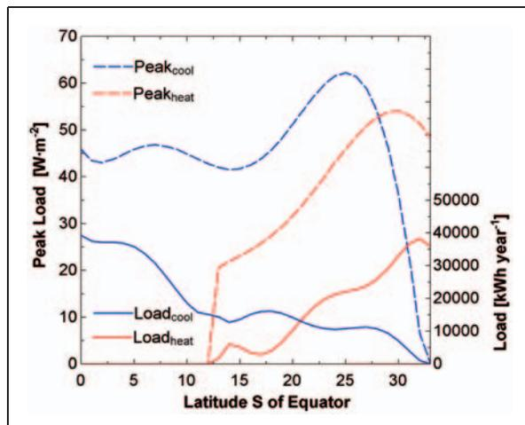
Figure 5. Latitudinal variation in Heating and Cooling Loads and Peak Capacity.
