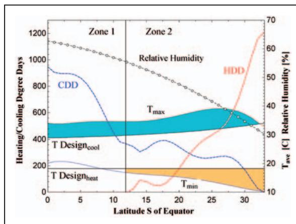
**Figure 2.** Latitudinal degree-day and temperature profiles for Africa based on NASA meteorological dataset. The design cooling temperature is based on Steadman's humidex.
