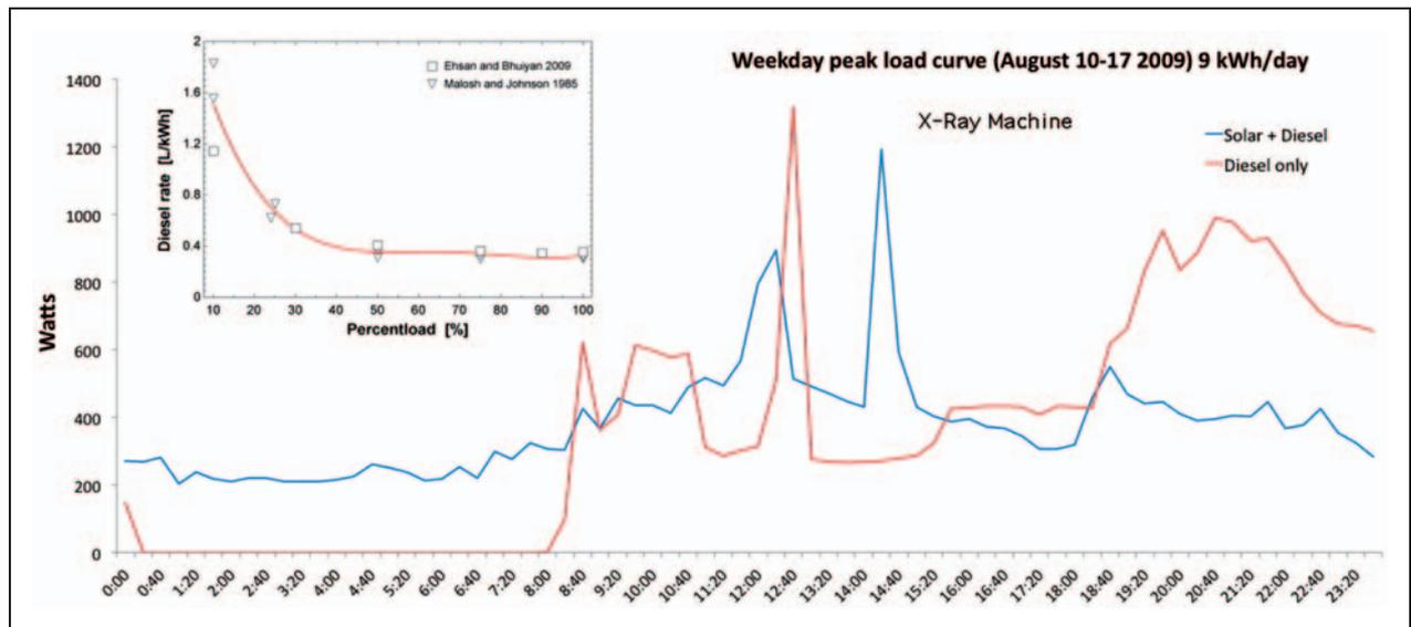
Figure 4. Measured PV and diesel clinic loads with part load fuel economy derived from Refs. 55 and 56.
