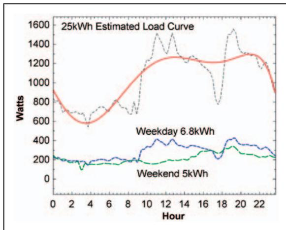
**Figure 3.** Measured and estimated health clinic load profiles. Average weekday (blue) and weekend (green) load curves are extrapolated to fit the load curve corresponding to the estimated target of 25 kWh day<sup>-1</sup> (red).
