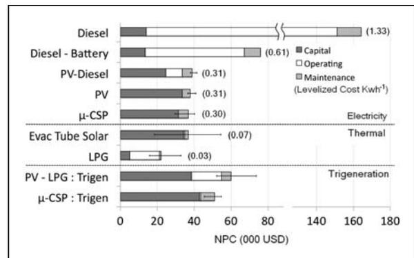
Figure 6. Net Present Cost (NPC) of distributed generation technologies meeting a typical clinic specification (25 kWh<sub>e</sub>, 118–139 kWh<sub>e</sub>·day<sup>-1</sup>, 330 days·year<sup>-1</sup>). Latitudinal variance due to thermal loads is indicated by bars where appropriate.
