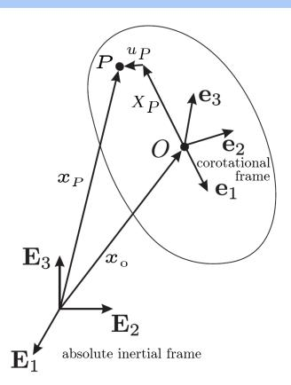
Kinematics of a superelement
