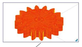
Simulation of unilateral contact between superelements (MATLAB)
