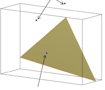
Projection point inside the surface element → active contact
