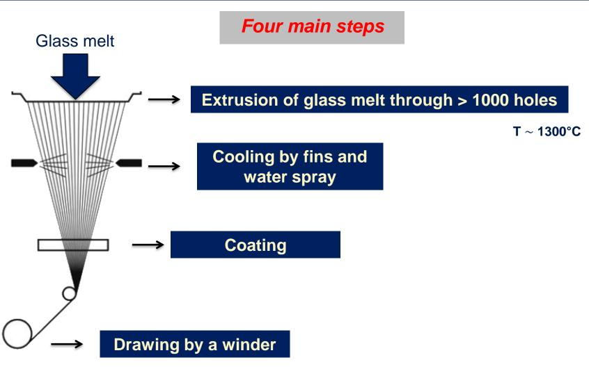
(20 m/s  $\rightarrow$  ~10 µm fibers diameter)
