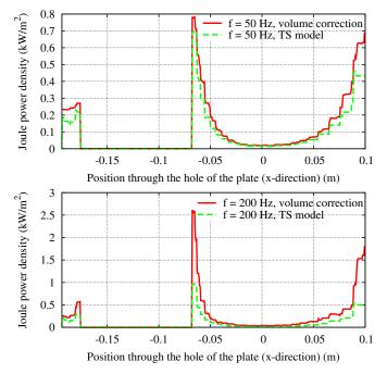
Fig. 6. Joule power loss density for TS model and volume correction through the hole (d = 19 mm).
