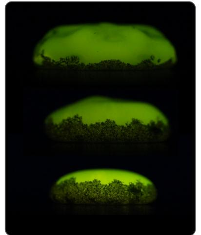
Fig. 2: Evaporating Leidenfrost droplet in which basalt grains were introduced.
