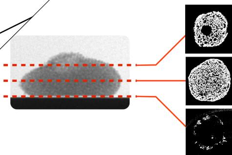
Fig. 7: X-Ray microtomography of the aggregation of glass beads after complete evaporation of the water.
