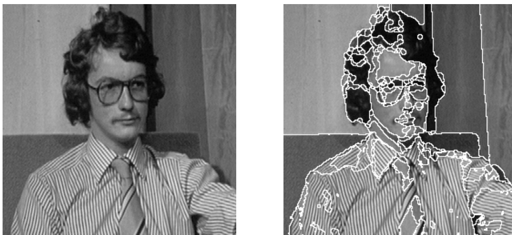
Figure 4: Final result of the segmentation process. All the shown parts of the shirt in the right-hand image have been detected as textures. The algorithm considers all the other regions as flat regions.
