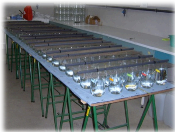
Fig. 2.1: Exposure beakers randomly exposed in the experimental room for the range finding test. Colours of the stickers correspond to chemicals.
