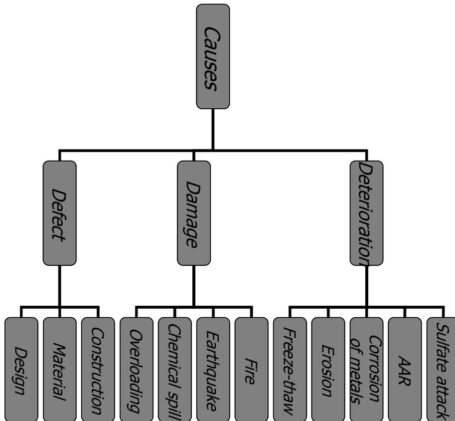
Figure 6: causes of concrete degradation
