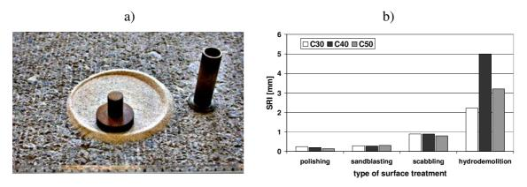
Figure 9: sand patch test (a) and examples of Surface Rough Index after different surface treatments (b) (Piotrowski *et al.*, 2007)
