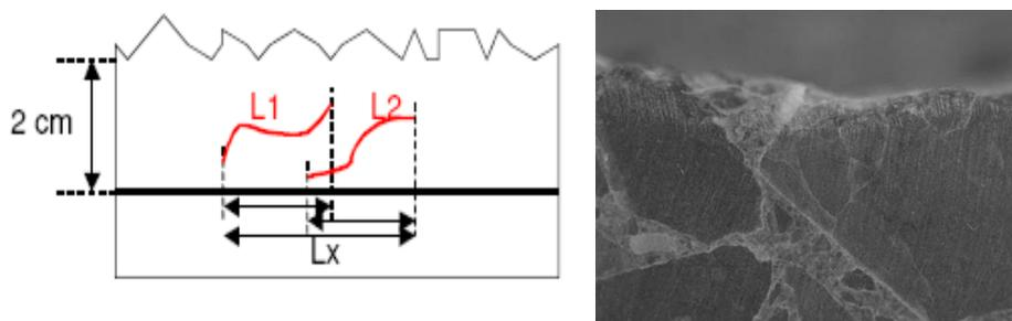
Figure 11: evaluation of the length ( $L_i$ ) of the cracks and their projection on horizontal reference ( $L_x$ )
