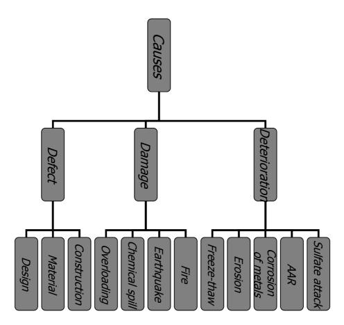
Figure 6: causes of concrete degradation
