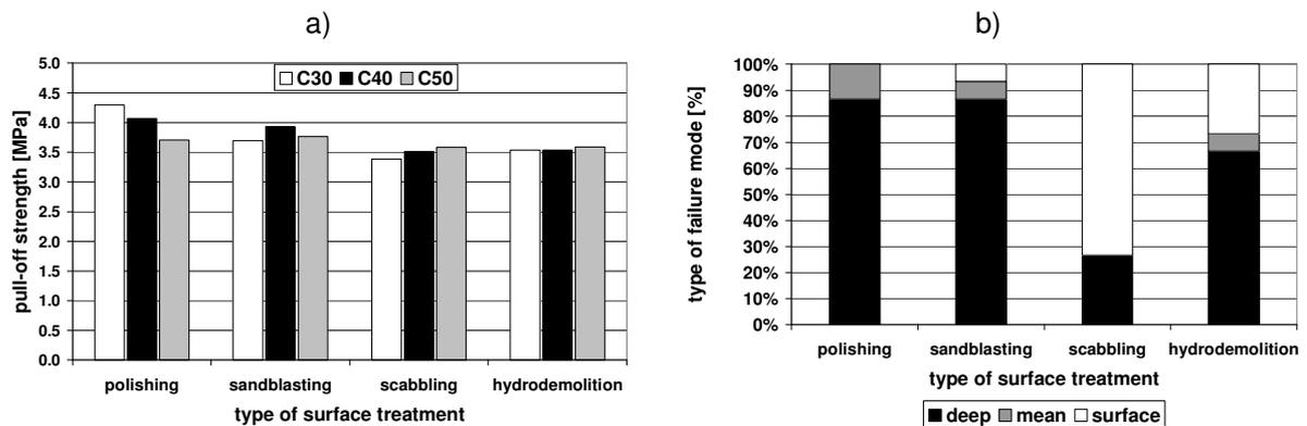
Figure 13: Pull-off cohesion test results (a) and type of failure mode registered (b) (Piotrowski *et al.*, 2007)
