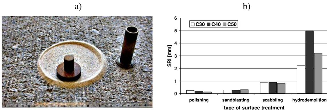
Figure 9: sand patch test (a) and examples of Surface Rough Index after different surface treatments (b) (Piotrowski *et al.*, 2007)
