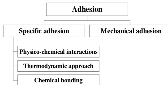
Figure 7: principles of the theory of adhesion.
