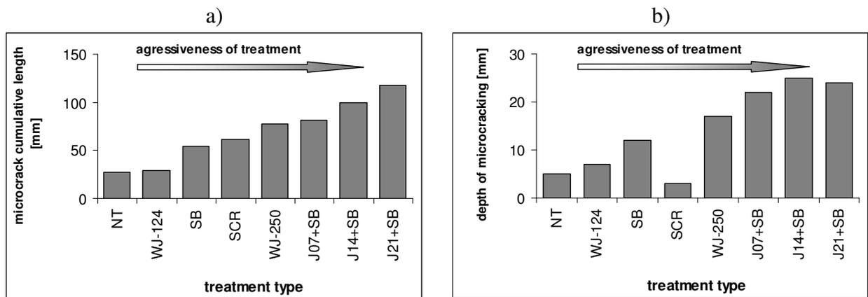
Figure 12: the length ( $L_i$ ) of the cracks (a) and depth of microcracking (b) against type of concrete surface treatment: NT – no treatment; WJ – water jetting – pressure 250MPa; SB – sandblasting; SCR – scabbling; J+SB – jack hammering of weight 7,14,21 kg + sandblasting (Czarnecki *et al.*, 2007)
