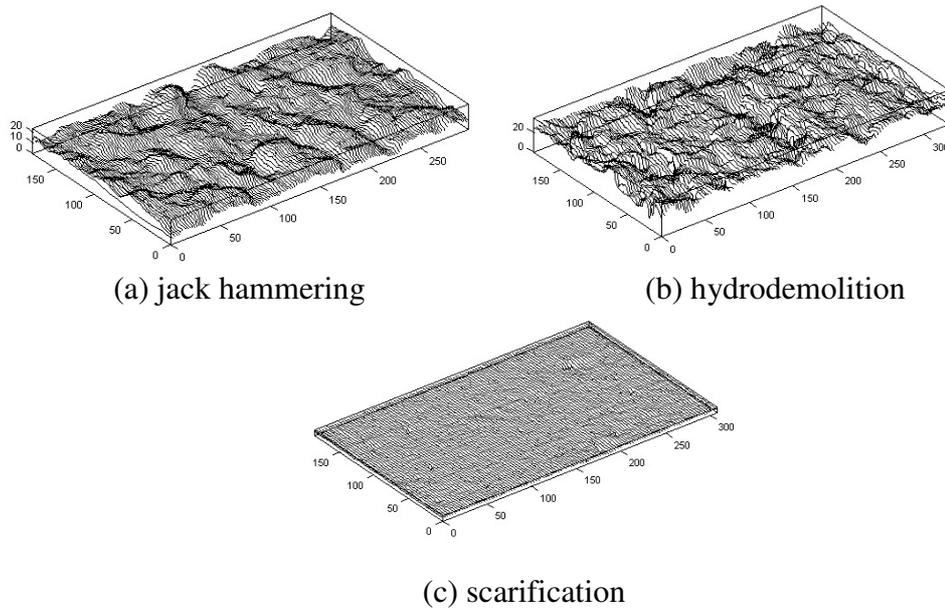
Figure 10: 3D-view of concrete substrate after different surface treatment (Courard, 2002).
