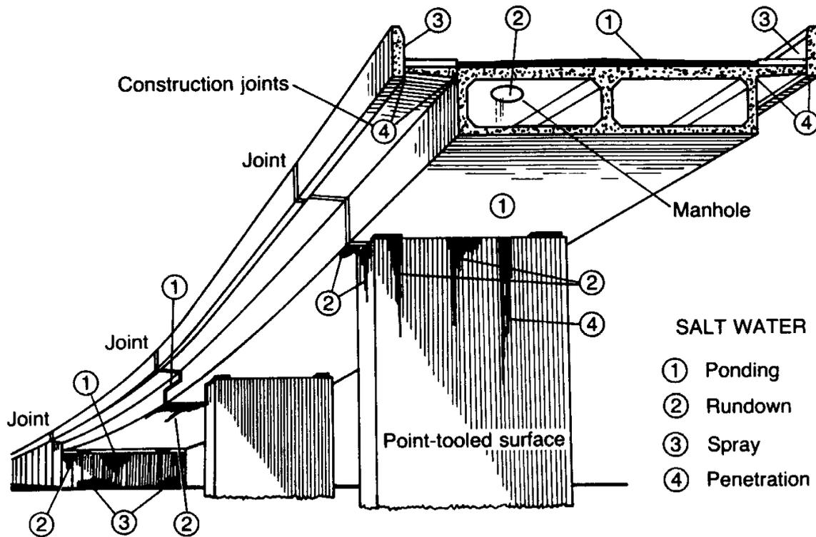
Figure 1 : typical zones of chloride ions attack (Pritchard, 1992)
