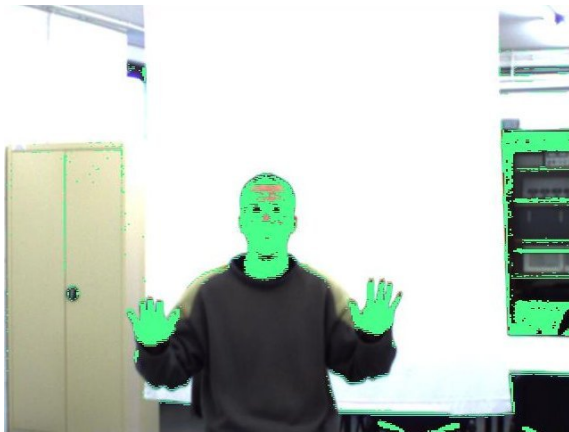
Figure 2: Skin thresholding in the YUV colorspace.
