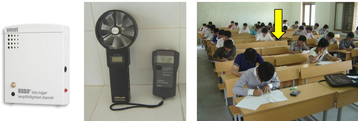
Figure 3-11: Measuring equipments used and class room arrangement in the survey (The downward arrow indicates the position of the data logger in the middle of the classroom).
