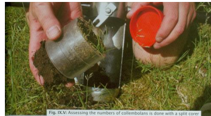
Fig. IX.V: Assessing the numbers of collembolans is done with a split corer which does not compress the soil. The collected soil sample is kept in a cylinder and brought to a high gradient extractor that dries out the soil. At which point the collembola leave the soil core allowing them to be collected, counted and identified (for more details see Chapter 8.2). (PHK)
