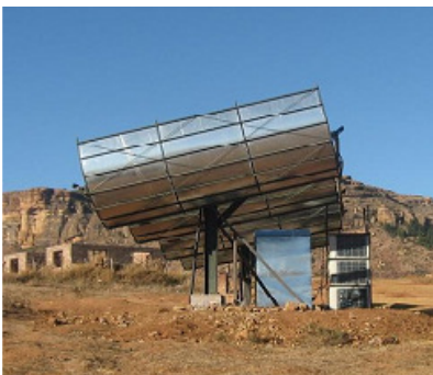
Figure 2 Solar ORC in field trials in Lesotho, southern Africa 2007 (Solar Turbine Group)
