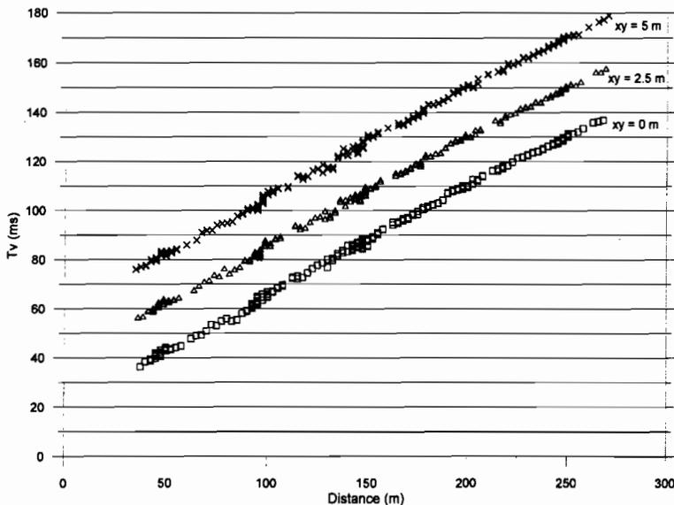
Fig. 5. Velocity analysis curves (line IV) computed by the GRM method for different  $xy$  values.
