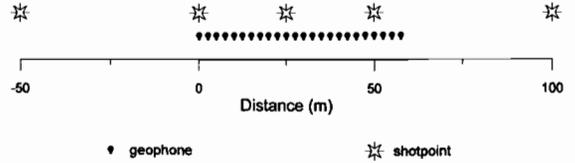
Fig. 2. Field configuration for the refraction profiles.
