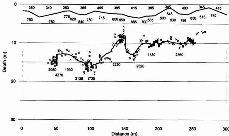
Fig. 7. Interpreted seismic cross-section along line IV.
