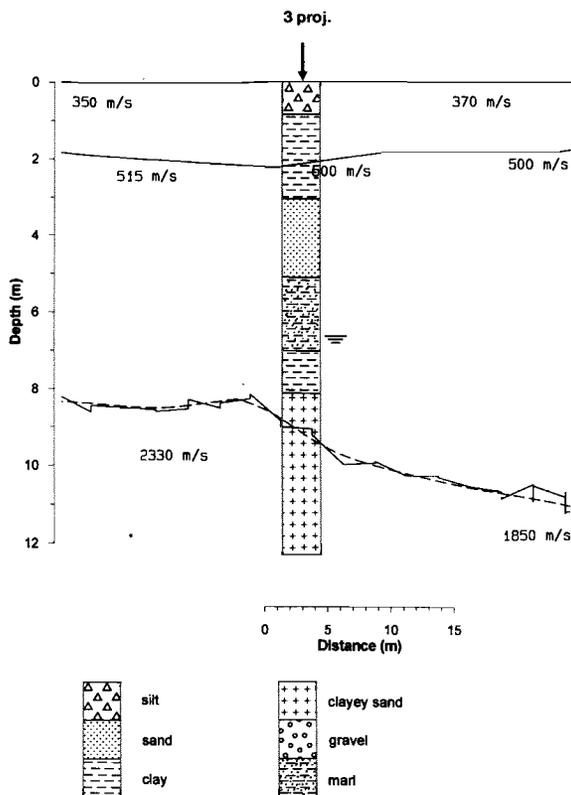
Fig. 8. Comparison between borehole P3 log and refraction data (line III).
