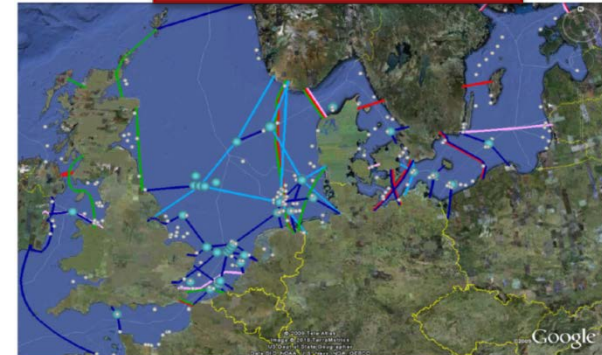
Offshore grid scenario 3: Wind-driven approach (blue = changes to base case, red = existing, pink = under construction, green = planned)
