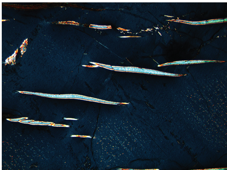
FIG. 2. Lamellae of zavaláite included in lithiophilite, La Empleada pegmatite, San Luis, Argentina (crossed polars, field of view 2.5 mm).
