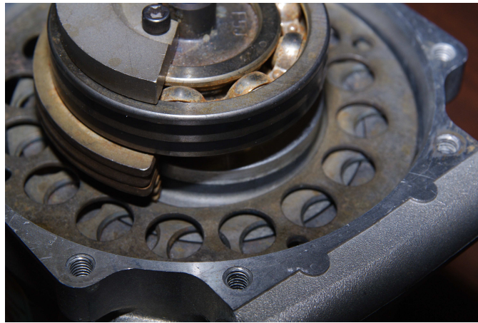
Figure 6.3. Internal structure of scroll compressor bearing system.
