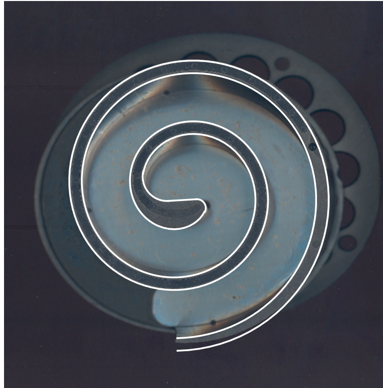
Figure B.2. Scanned Sanden Scroll orbiting scroll with overlaid curves.
