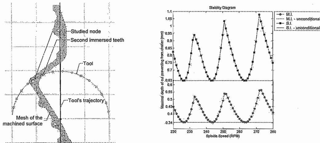
Figure 7; left: identification of the studied node. Right: Stability diagram for the two immersed teeth (MI) or with only the teeth on the studied node (SI).
