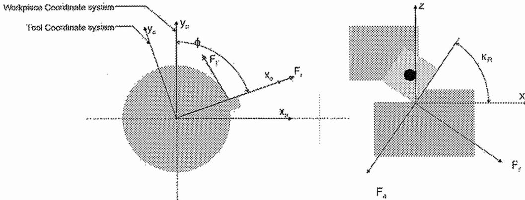
Figure 1; The two rotations.  $\kappa_R$  is the tool working cutting edge angle.
