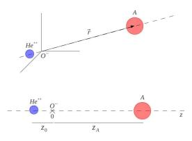
Figure 1: One-dimensional OHe atom polarized along the O<sup>--</sup>-A axis, denoted z.  $z_0$  is the distance between O and He and  $z_A$  is the distance of the A nucleus along the z-axis.
