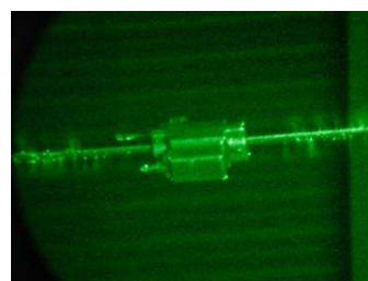
Ampacimon during heavy rain corona test at "Les Renardières" (France).
