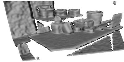
Figure 2: Range image captured by the Microsoft Kinect, filtered with our algorithm and displayed in 3D using MeshLab.
