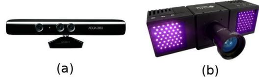
Figure 1: (a) Microsoft Kinect and (b) PMD[vision] CamCube cameras.
