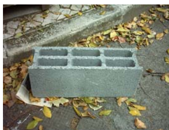
Figure 6 – Hollow concrete blocks used in the inner wall
