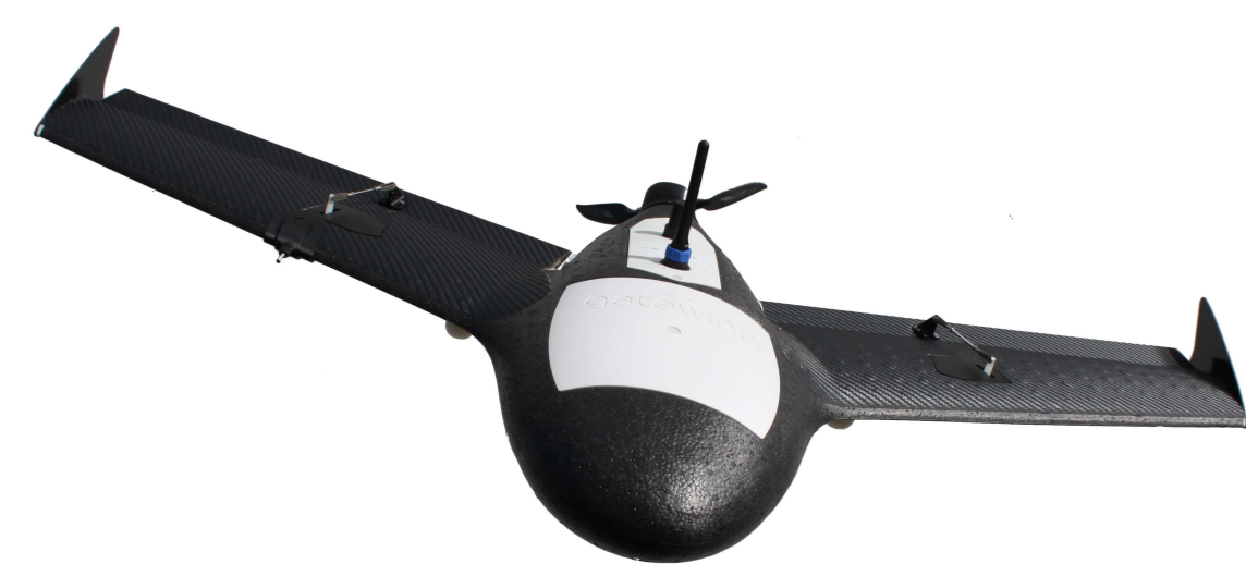
FIGURE 2: The Mini-Unmanned Aerial Vehicle used in this research. The X100 Gatewing is a fixed-wing of 2kg flying with an electric motor at the cruise speed of 80km/h. Its flight duration of 40 minutes enable to cover areas of more than 100 ha with high overlap (80%) at 250 m above ground level.
