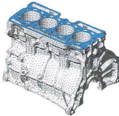
4-cylinder crankcase, 330000 dof, 839 retained nodes 515 sec.
