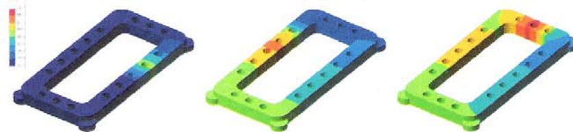
Figure 9: evolution of temperature from a thermal analysis when drilling respectively 2 nd , 11 th and 15 th holes in an aluminum sample
