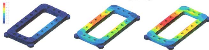
Figure 10: evolution of displacements from the mechanical analysis (same holes as figure 10); the part is clamped at each of the four corners
