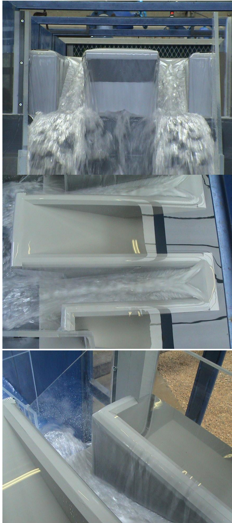
Figure X-10 Views of the scale model for a discharge corresponding to Q = 1.2 \text{ m}^3/\text{s}
