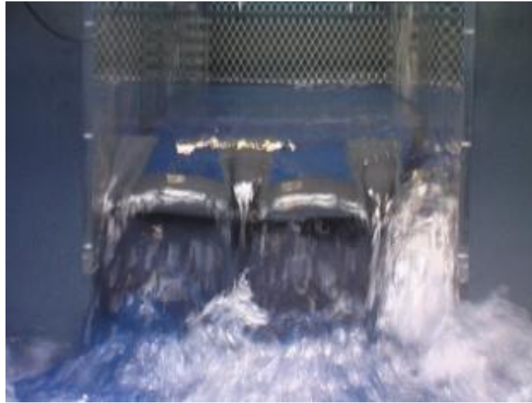
Figure VII-16 View of the downstream nappe aeration for H = 0.2 m and P = 0.1 m
