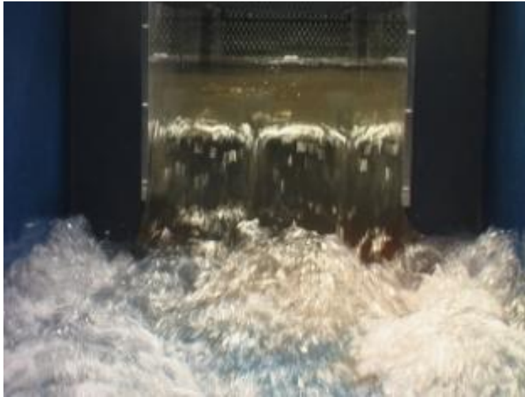
Figure VIII-25 No more air entrainment and leaping nappe on the PKW for H = 0.21 m and W_i/W_o = 2
