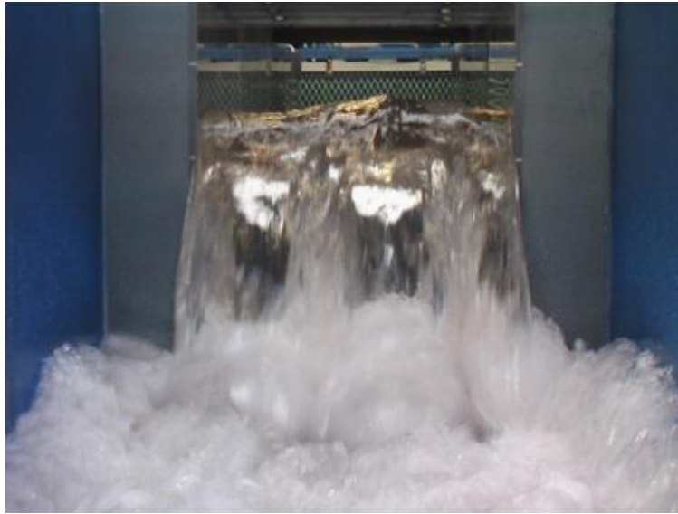
Figure VII-41 View of the transverse free surface variation for H = 0.24 m on variant 2 of model 3
