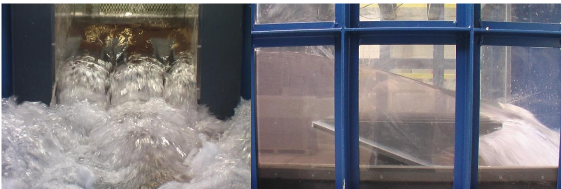
Figure XIV-22 PKW model 4 under a high upstream head ( H = 0.256 cm)
