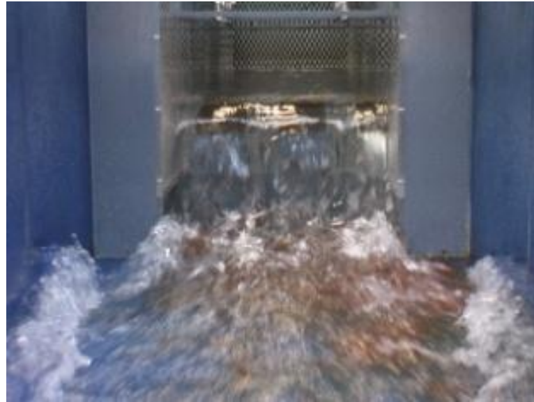
Figure IX-18 No more air entrainment and leaping nappe on the model with technico-economic height optimization for H = 0.155 m and B_o/B_i = \infty
