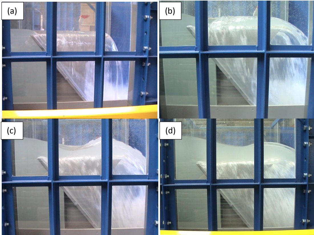
Figure IV-16 View of the outlet free surface variation with head: H/P = (a) – 0.1; (b) – 0.2; (c) – 0.35; (d) – 0.5
