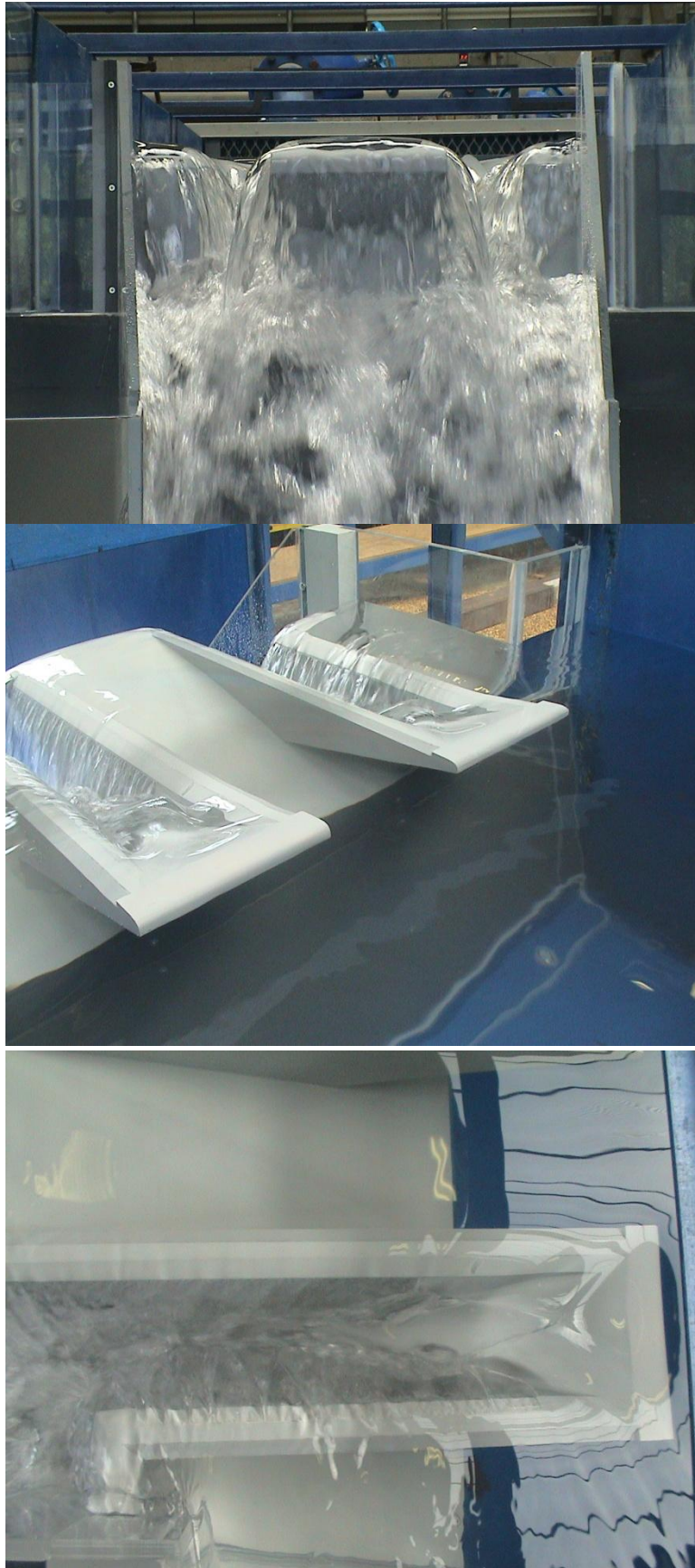
Figure X-9 Views of the scale model for a discharge corresponding to Q = 5 \text{ m}^3/\text{s}
