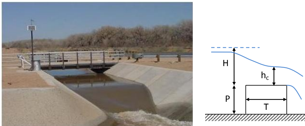
Figure II-2 Flow over a broad-crested weir
