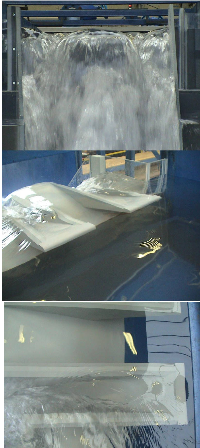
Figure X-8 Views of the scale model for a discharge corresponding to Q = 10 \text{ m}^3/\text{s}
