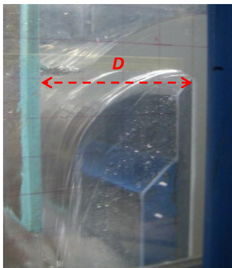
Figure V-5 Experimental sharp-crested weir influenced by a downstream vertical wall
