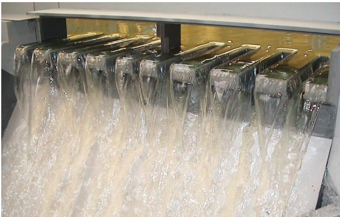
Figure XII-2 1:35 scale model of the first design for the Ravière PKW – Q = 24 \text{ l/s}
