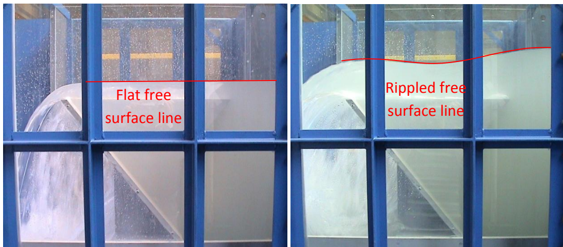
Figure IV-13 Surface line profiles for low and high heads ( H/P = 0.15 and 0.35 )
