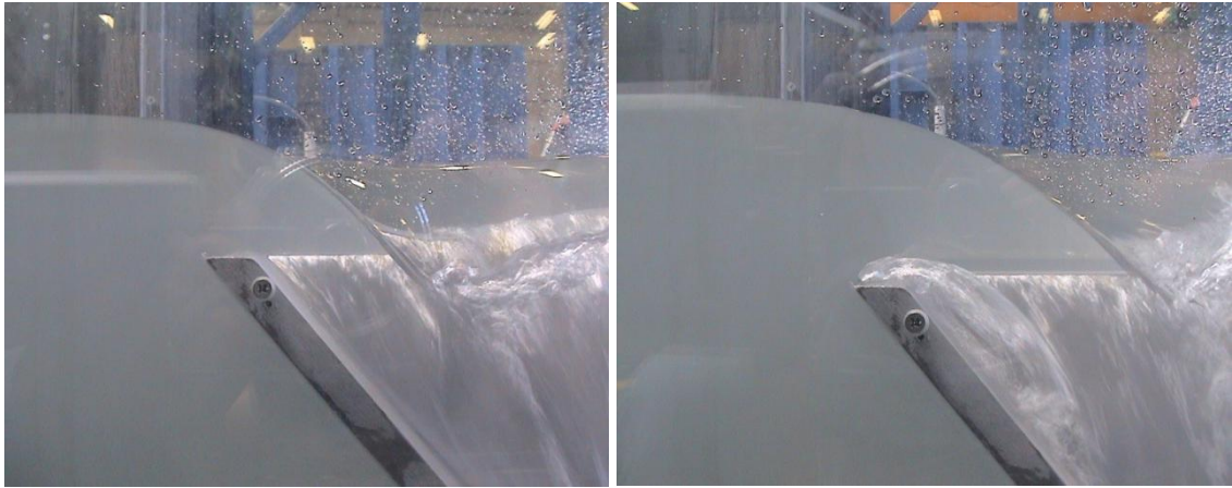
Figure IV-7 Transition from a clinging to a springing nappe on the upstream crest
