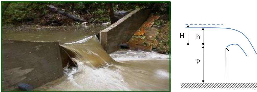
Figure II-1 Flow over a sharp-crested weir
