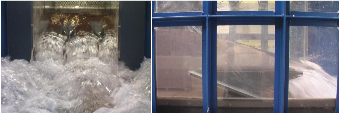
Figure V-9 PKW model 4 under a high upstream head ( H = 0.256 cm)
