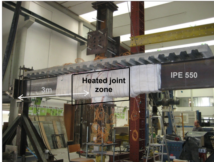
Figure 20: Heated connection zone using Ceramic Pad Heating elements
