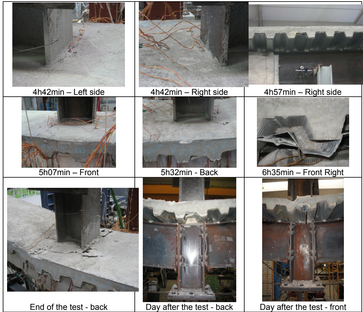
Figure 211: Evolution of the concrete crushing
