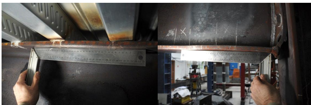
Figure 152: Local buckling of the flanges from the right beam (view from the back)
