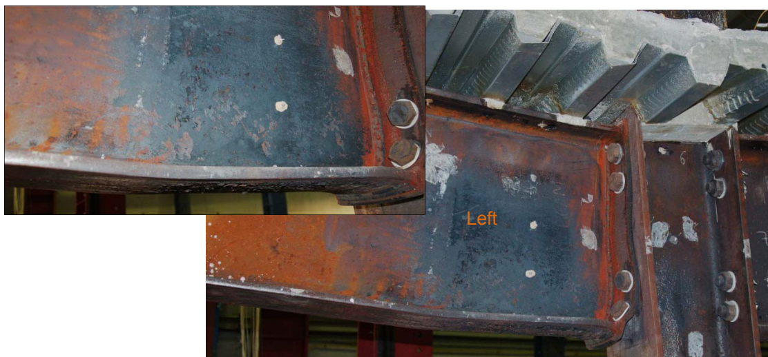
Figure 120: Deformation of the beam bottom flange (left side) – Front view
