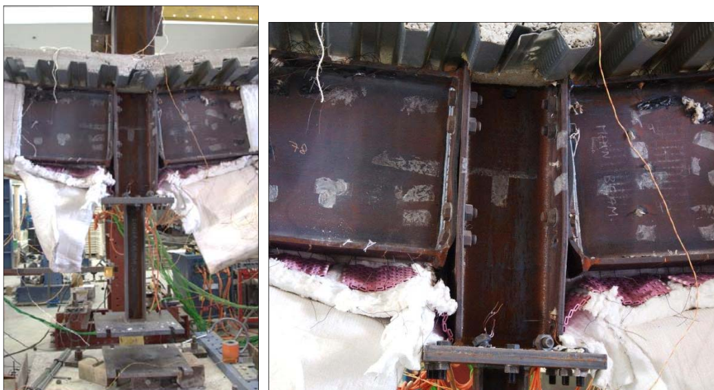
Figure 90: Final deformation of the sub-frame at the end of the test
