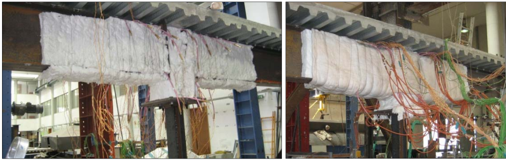
Figure 22: Thermal insulation of the ceramic pad heating elements (rock-wool of density 128\text{kg/m}^3 )
