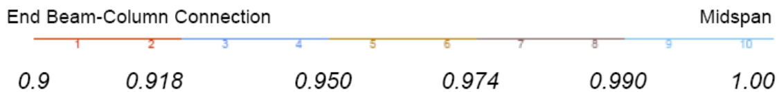
Figure 10. Coefficients of reduction of the temperatures along the beam used in SAFIR
