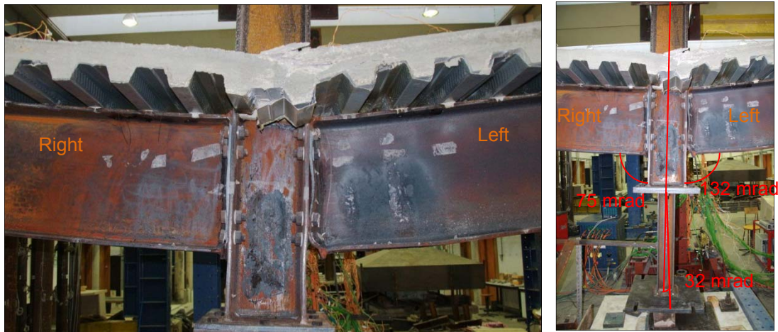
Figure 119: Final deformation of the sub-frame under sagging bending moment (back view)
