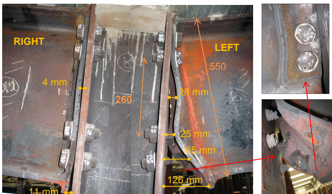
Figure 278: Deformations of the joint (view from the front side)
