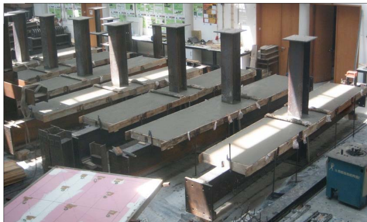
Figure 19: Specimens after the concreting of the composite slabs, at the floor level
