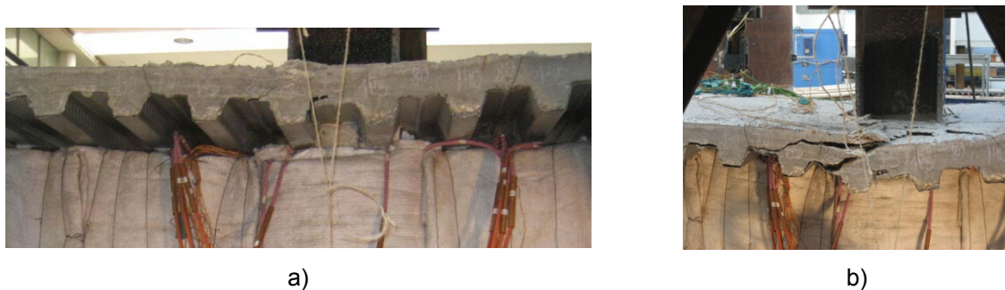
Figure 228: Concrete crushing on the back side of the slab at vertical displacement equal to: a) 158 mm; b) 214 mm
