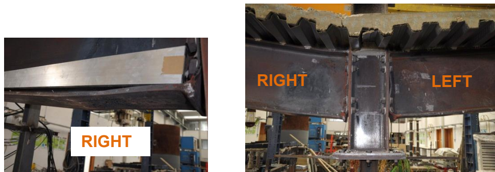
Figure 192: Beam rotation near the joint
