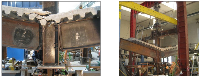
Figure 1. Final deformation of the tested structure (test 6)
