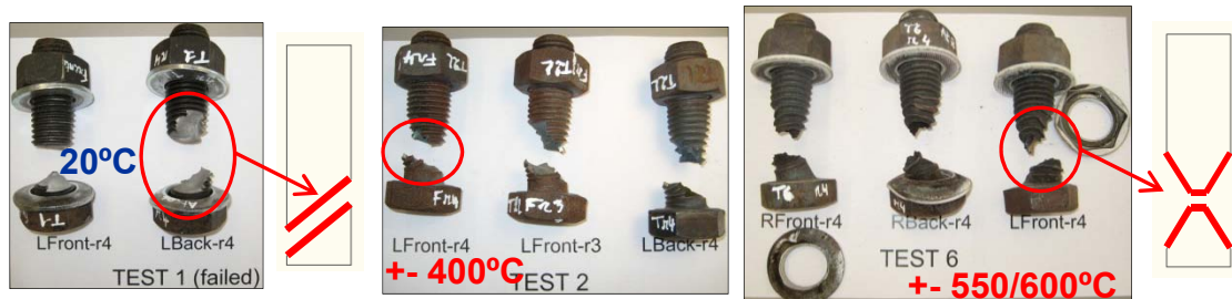
Figure 317: Bolts failed in tests 1, 2 and 6
