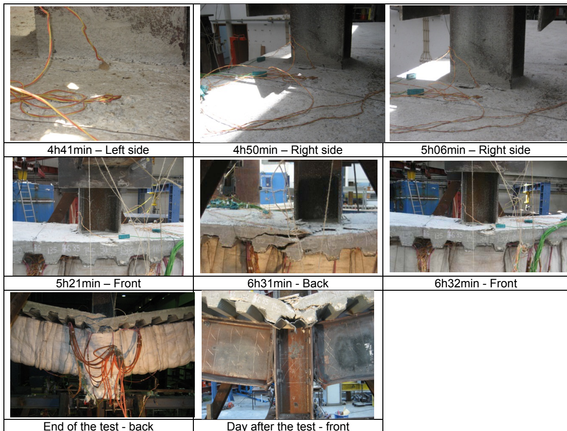
Figure 256: Evolution of the concrete crushing
