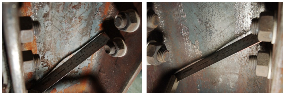
Figure 116: Local buckling of the column web on the bottom part (level of the bolt rows 3 and 4) under hogging bending moment
