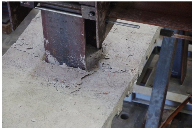
Figure 89: Crushed concrete slab at the end of the test
