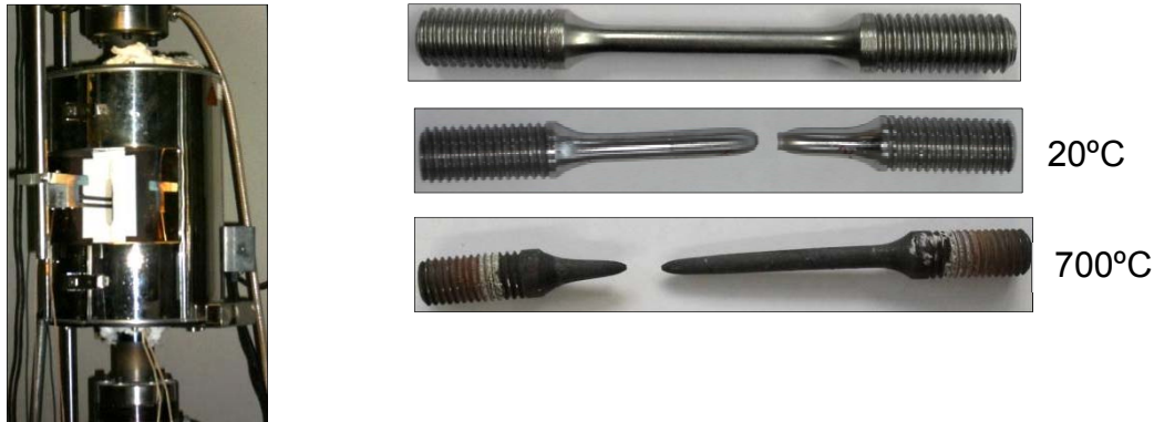
Figure 37: Testing furnace and steel coupons before or after the tests
