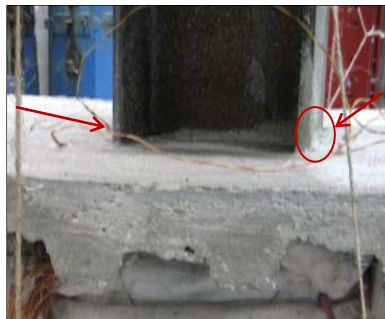
Figure 146: Concrete crushed against the column flange
