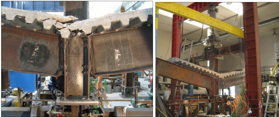
Figure 314: Final deformation of the tested structure (test 6)
