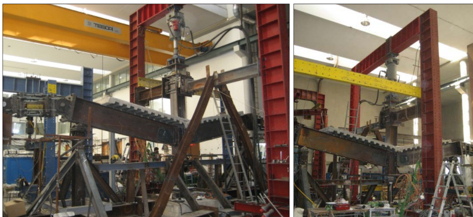
Figure 271: Final deformation of the sub-frame the day after the test
