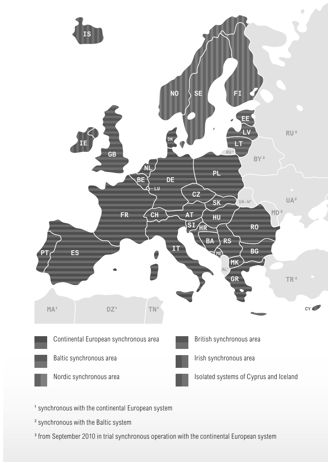
Figure 2.6: European map with indication of the interconnected ENTSO-E system members (2011); continental European synchronous area is represented in the PEGASE system
