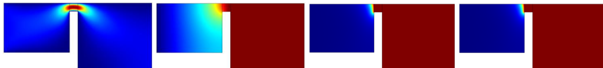
Figure 7: From left to right: the velocity field ( 0 - 0.0236 \text{ m/s} ), the electron concentration ( 0 - 2.297 \cdot 10^{-3} \text{ mol/m}^3 ), the O radicals concentrations ( 0 - 1 \text{ mol/m}^3 ) and the CO concentration ( 0 - 1 \text{ mol/m}^3 )
