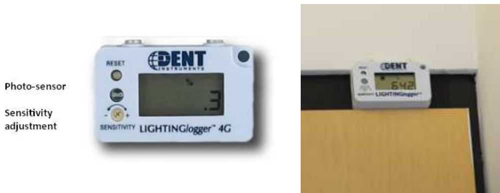
Figure 28: Lighting operating time logger (left) installed in the elevators area (right)
