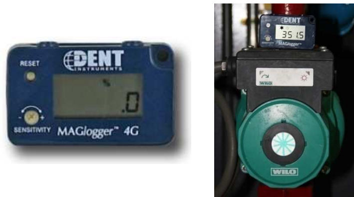
Figure 29: Magnetic field logger (left) installed to monitor the operating time of a pump (right)
