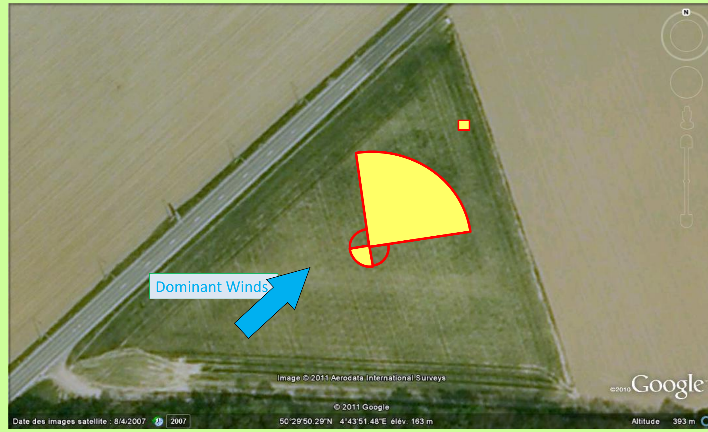
Picture I : Aerial view of the experimental design fitted on the field. Note upwind and downwind areas and the single plot on the 45° ray, at 128m from the introduction point.
