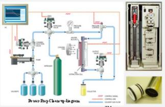
**Clean-up:** The automated Power-Prep<sup>TM</sup> system (FMS Inc.) was used for sample clean-up [1,2]. Both PLE and clean-up systems were connected to on-line evaporation devices that ensured proper solvent reductions.
