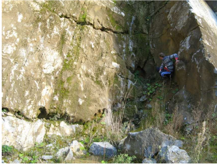
Picture 6: SE view (perpendicular to S_0 ) of the bottom of the Mercier quarry. Two major karstic conduits are presented here. Their thicknesses can be decimetrical to metrical and therefore, such karstic conduits are major preferential paths for groundwater flow.
