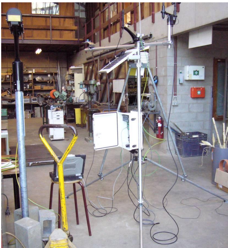
FIGURE 7. STATION METEO ET DISDROMETRE
