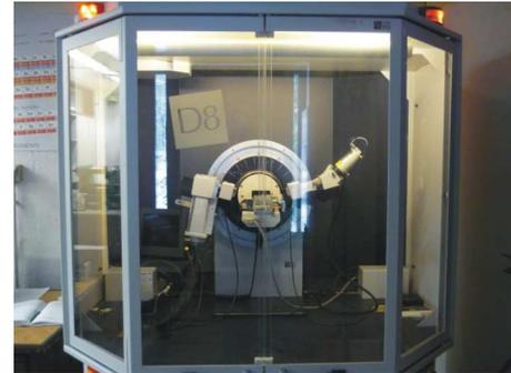
Fig. III.4. Appareil de diffraction des rayons X Bruker AXS D8 Advance.
