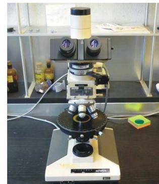
Fig. III.1. Microscope polarisant Olympus BH-2
