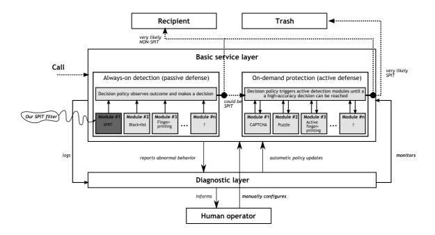
Figure 5: A hierarchical and modular SPIT prevention system. The SPRT-based SPIT filter we propose in this paper is one particular module in the always-on component of the basic service layer.
