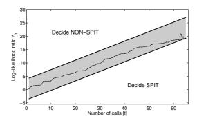
Figure 3: An example run of SPRT. The log-likelihood ratio  $\Lambda_t$  starts at t=1 in the region between the decision boundaries and, with each new sample observed from the unknown source, performs a random walk over time. Eventually it will cross over one of the decision boundaries and either enter the region marked "decide SPIT" or enter the region marked "decide NON-SPIT".
